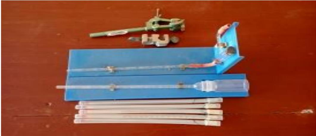
Gambar: Termometer suhu tanah, respirometer, potometer, dan boshead.
