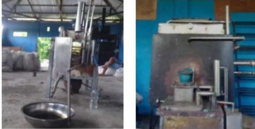
Figure 7. Pyrolysis Machine for Processing Plastics into Fuel with Capacity of 10 and 50 kg
